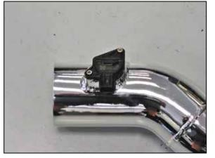
16. Install the mass air sensor into the  $K\&N^{\otimes}$  intake tube and secure with the provided hardware.
