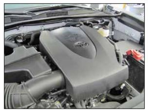
2. Lift up the engine cover to dislodge it from the mounting studs and then remove it from the vehicle.
