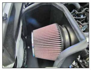
21. Install the K&N<sup>®</sup> air filter onto the filter adapter and secure with the provided hose clamp. NOTE: Drycharger<sup>®</sup> air filter wrap; part # 22-8049DK is available to purchase separately. To learn more about Drycharger<sup>®</sup> filter wraps or look up color availability please visit http://www.knfilters.com<sup>®</sup>.
