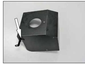
9. Install the provided heat shield bracket (07958) onto the K&N<sup>®</sup> heat shield as shown.
